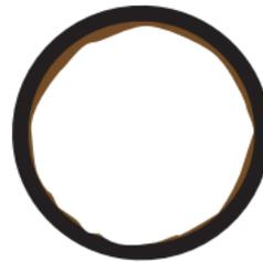
BioOne treated drain line after 8 weeks
